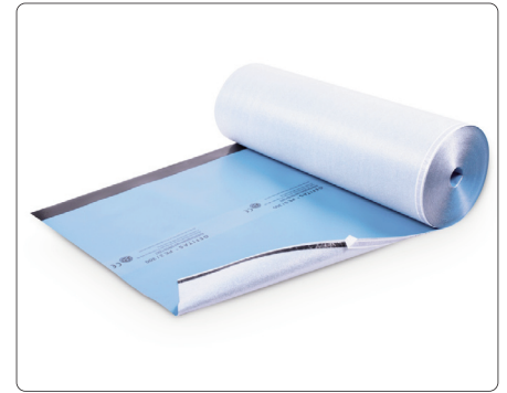
Sealing roll Moisture barrier with adhesive strip to protect insulation and floor surfaces against rising damp according to DIN/EN, roll size 1.25 m x 40 m; thickness: 3 mm foam backing + 0.3mm PE film = 3.3mm 080017-50 50 m 2 /roll
