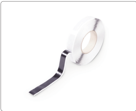
Sealing tape Self-adhesive moisture barrier to protect insulation and floor surfaces against rising damp according to DIN/EN, roll size 0.02 m x 15 m; thickness: 3 mm foam backing + 0.3mm PE film = 3.3mm 080017-15 15 m/roll
